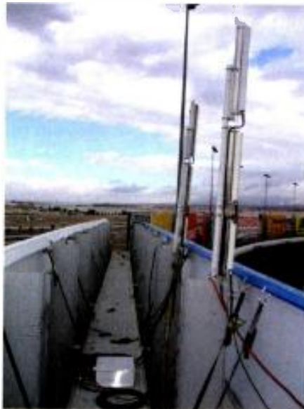
The receive boxes (seen at the lower left, antenna upper right at track side) work within the 1.4GHz to 1.5GHz and 2GHz to 2.5GHz spectrum and, for NASCAR events, are located at strategic points around a race track.
