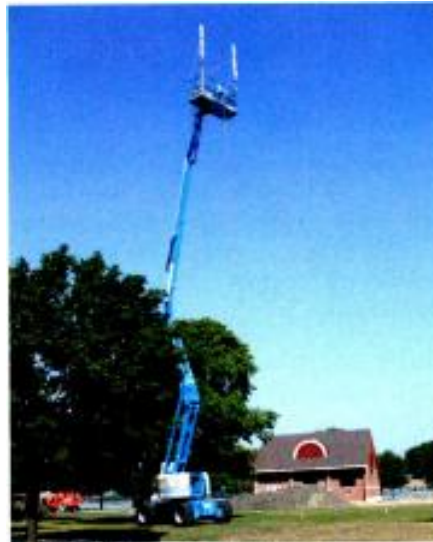
BSI's "portable" RF infrastructure can include receive sites mounted on a series of booms and works with any DVB-T compliant wireless camera or mic transmitter.
