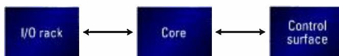
Figure 1. Modern consoles have found a superior phenotype in a digital, three-block design. The design removes the physical constraints of a single-box console and means every part of the console is customizable, upgradable and expandable.
