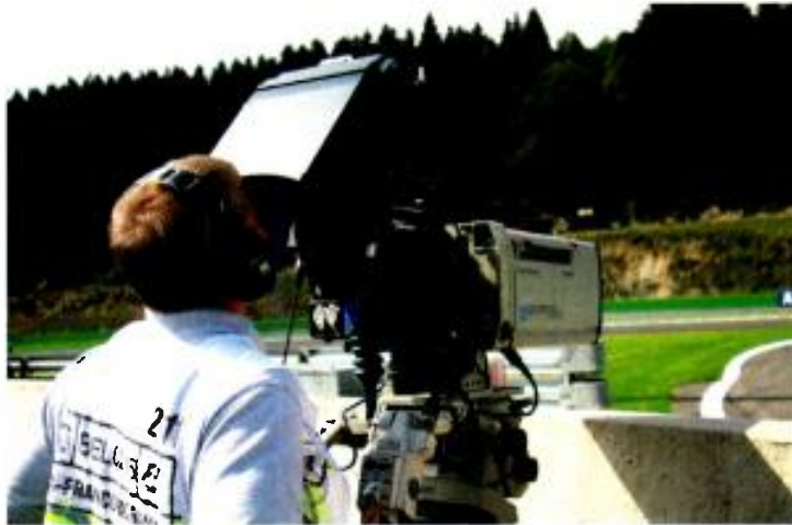
With CMOS technology, the Vision Research-based camera system can acquire images in incredibly high frame rates and can be accurately matched to standard HD cameras.
