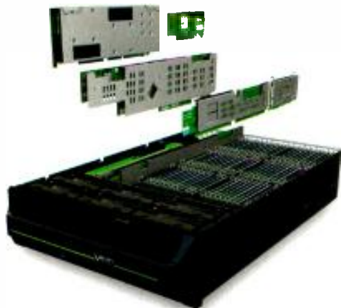
Each rack in the Violin Memory 6000 series has the potential to deliver 12 million IOPS and 48GB/s of bandwidth.
