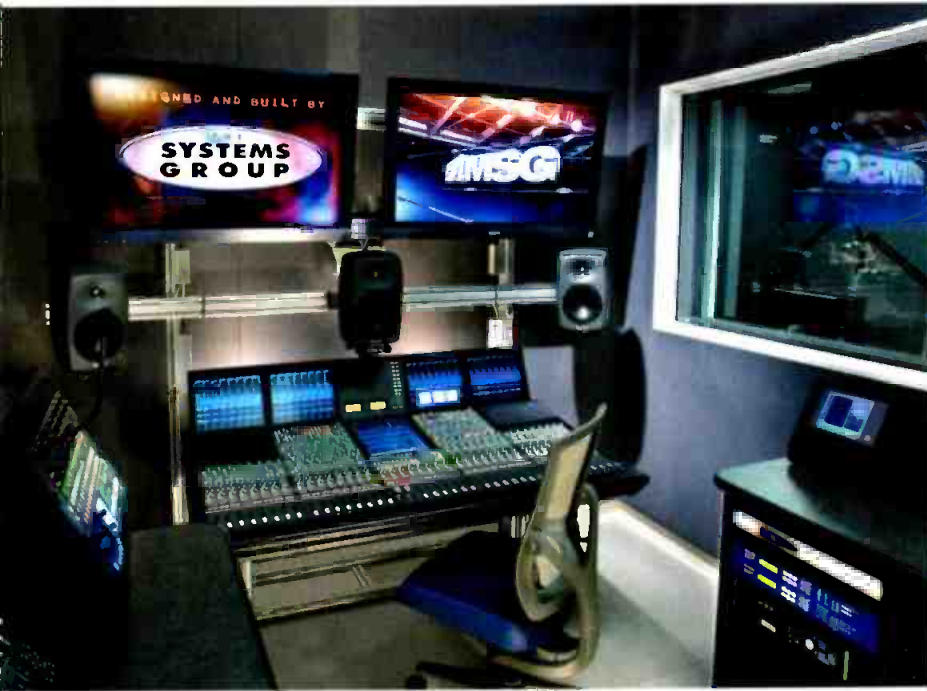
The "multipurpose" room at MSG Media's facility, in New York, houses the Solid State Logic C100 HDS console. The board's primary use is for live audio mix, voice-over and SAP.
