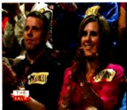
"Slice order" errors in MPEG transport streams can cause blockiness and other picture distortions.
