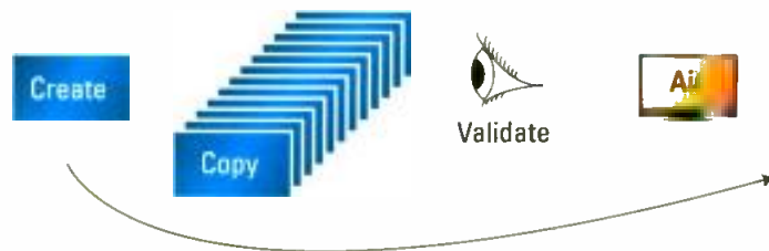
Figure 1. There are four basic steps common to contemporary graphics workflows: creation, versioning (copy), verification (validate) and playout (air).
