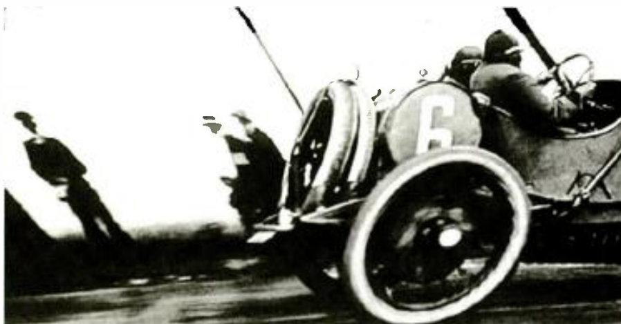
Figure 1. This rolling shutter artifact caused the car wheel to appear oval.
