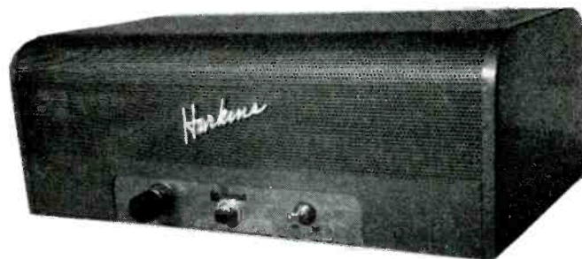
The HARKINS Multiplex receiver which features an I.F. amplifier operating at 23 Mc. for high phase linearity and a subcarrier filter that enables full 10 Kc deviation.
