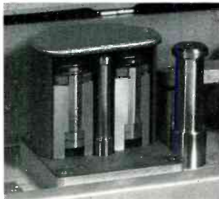
Changes in VR-1000 audio head assembly reduce oxide accumulation. New cue track erase and record-playback heads trace track on lower edge of 2-inch tape.
