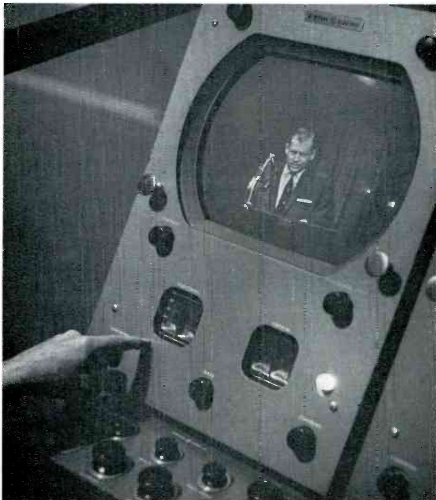
Engineer points to the wave form monitor which indicates the brightness values from black to white in the scene being telecast.
