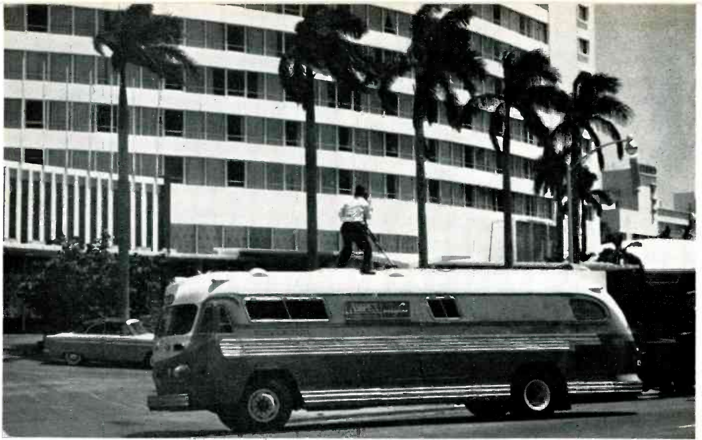
The Ampex Videotape Cruiser wheels into the driveway at the Fontainebleau Hotel, Miami Beach, during the taping of a special telecast for WPST-TV (Channel 10), Miami. Note cameraman in action atop the Videotape Cruiser. A completely self-contained, mobile tape studio with two TV cameras, power unit and Videotape television recorder, the Ampex unit was in Miami for the Society of Motion Picture and Television Engineers convention. The special telecast recorder with the Videotape Cruiser featured a tour of Miami Beach's famous hotel row.
