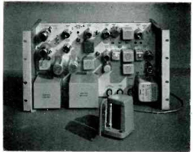
Associated equipment for the VR-1000 includes 2-inch automatic erase head. Electronics chassis mounts in front of console, provides current and amplification both for cue track and erasing function.
