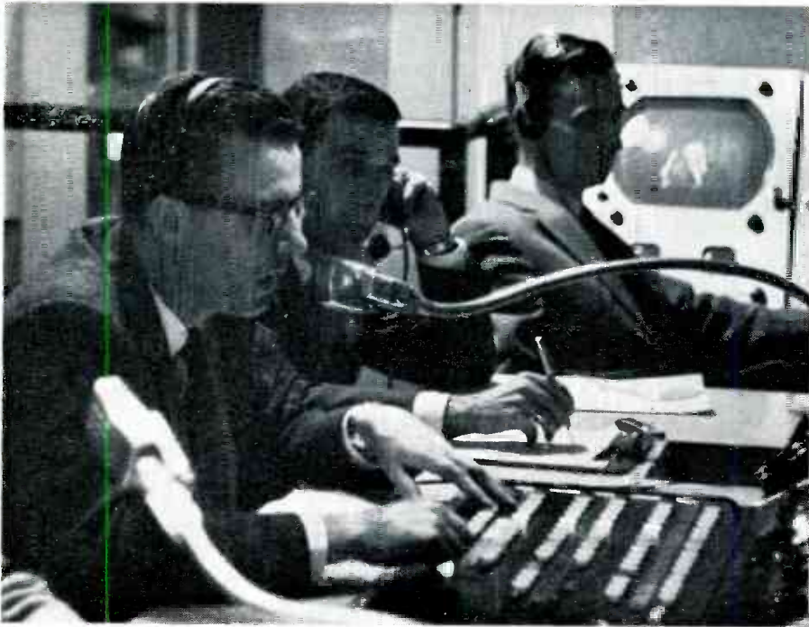
ABC-TV engineer at the switcher coordinates the video elements of the "Operation Videofilm" telecast.
