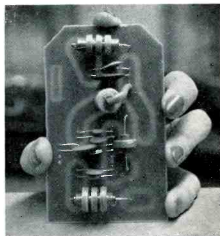
Fig. 2. Band pass filter used in receiver is assembled on an etched circuit board. The etched circuit shows through from the rear due to translucence of material.
