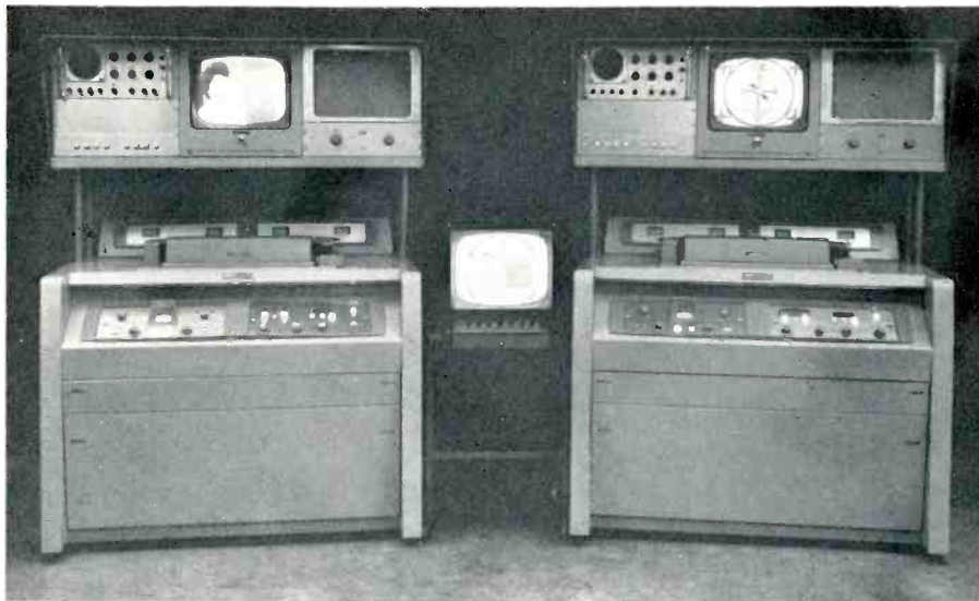
NEW VIDEOTAPE* DEVELOPMENT — By means of the new Inter-Sync device developed by Ampex for its Videotape recorder, the playback outputs of the two VTRs shown here are synchronized precisely for feed to a third monitor.
