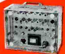
1073-D1 SINE SQUARED (SIN 2 ) — SQUARE WAVE GENERATOR
