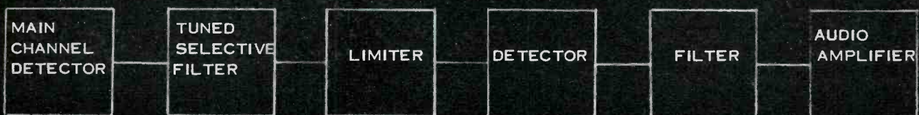
Figure 2. Block diagram showing stages used in selective filtering method of subcarrier recovery.
