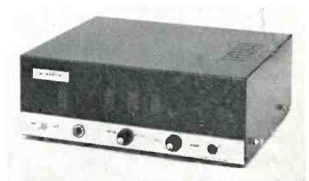
Figure 7. McMARTIN multiplex receiver utilizing the heterodyne principle.
