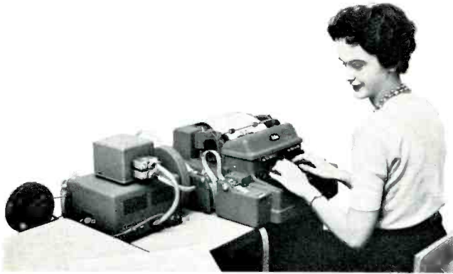
Figure 2. Traffic director types schedule and simultaneously punches control information on paper tape.
