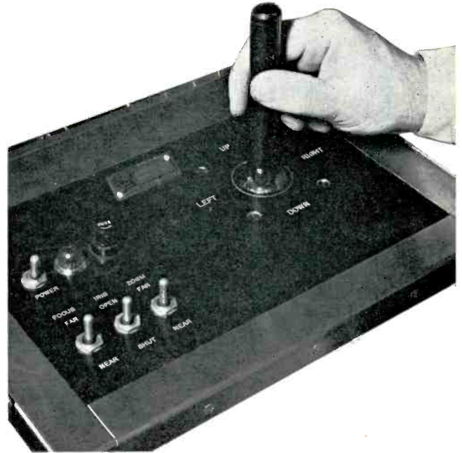
Figure 8. A "Joy-Stick" is used for pan and tilt. Toggle switches are used for zooms and focus.
