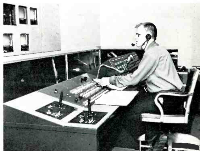
Figure 12. The director's control room contains a duplicate set of switching and remote camera control facilities.
