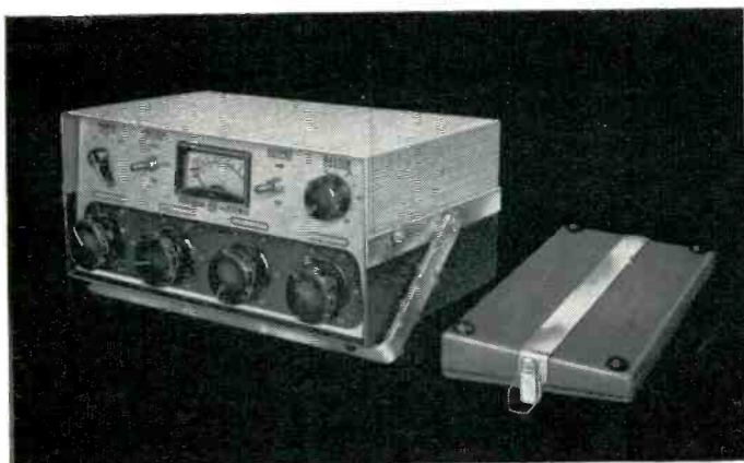
Carrying handle functions as base to position unit for most convenient operating angle.
