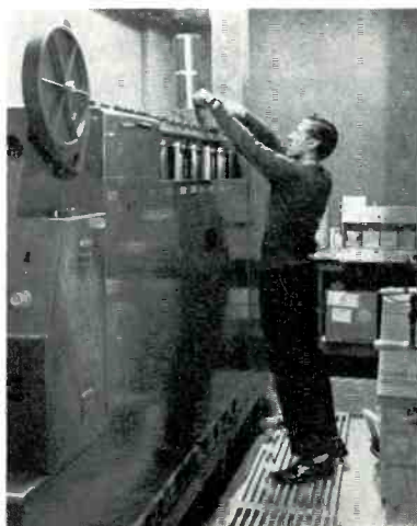
Figure 7. Two RCA television recorders are located in the Master Control Room directly behind the switching position. The machines are remotely controlled from any switching position.
