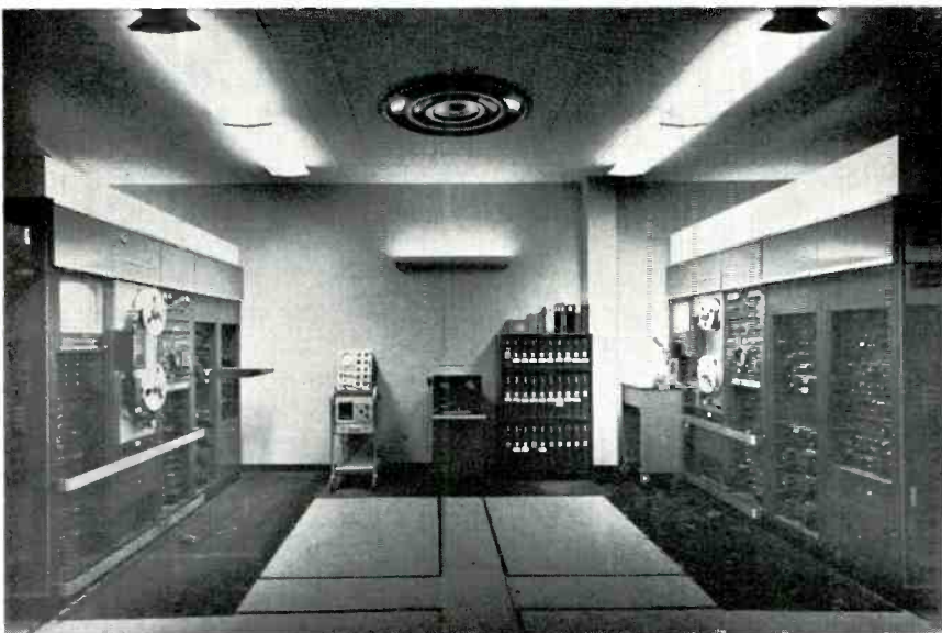
Figure 7. Two RCA television recorders are located in the Master Control Room directly behind the switching position. The machines are remotely controlled from any switching position.
