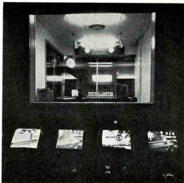
Figure 4. A view of the audio control for Studio B from the Master Control. The Audio Control Room is equipped with the latest all transistor two channel console, two turntables, video monitor, and remote controls for three automatic tape machines.
