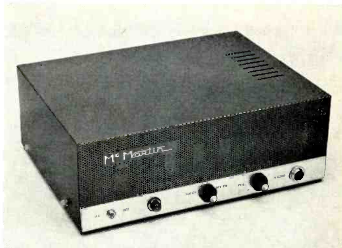
Figure 3. Complete Multiplex receiver including MT-12 selective muting unit.
