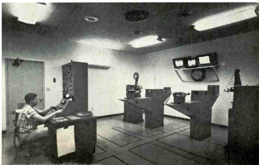
Figure 5. The Telecine Center showing the complete vidicon film chains, film projectors, slide projectors, and engineer's control desk. Except for live programming all audio is controlled from this point. In the two racks can be seen the automatic tape machines and the automatic station break programmer designed and built at WJXT.
