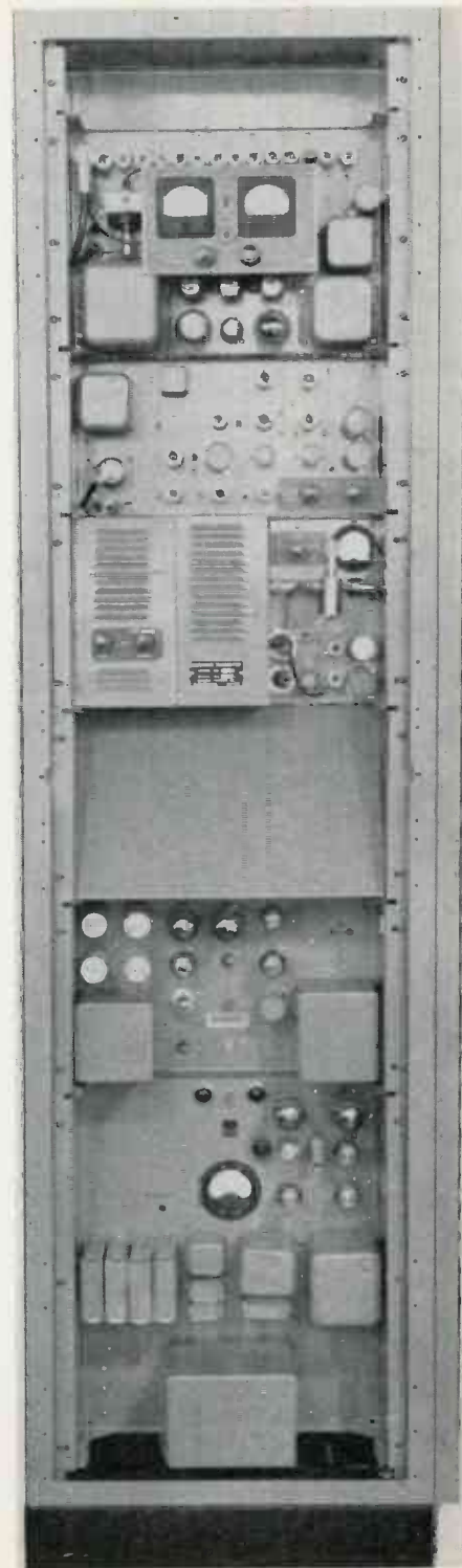
Fig. 2 — Sarkes Tarzian M/W Equipment, Model MWF-1C, long-range microwave relay.
