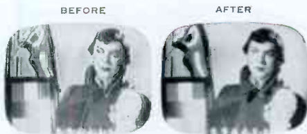
Photos, taken a few seconds apart, show how the Model 20/20 cleans up smears, overshoots, ringing and other waveform defects.
