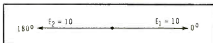
Fig. 6. Diagram of two opposing vectors. zero, since it is the reference tower. If the current ratios and end tower phases are made equal, the equation can be simplified. This is due to the vertical components of the vectors cancelling out:
