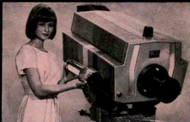
This 4½-inch image orthicon (black tube) is used in the separate luminance channel to sharpen the color picture and to assure a high-quality monochrome picture.
