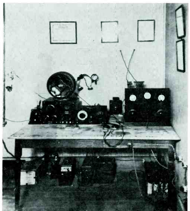
Fig. 3. A composite transmitter in use in 1919. Note the chemical rectifier on the floor at the right end of the table.
