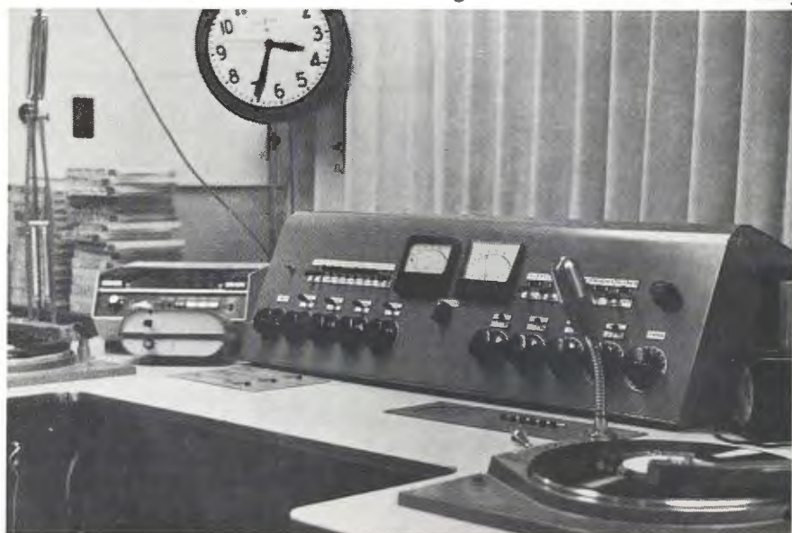
Fig. 5. Another student-built dual-channel audio board is in use at KCSM-FM.
