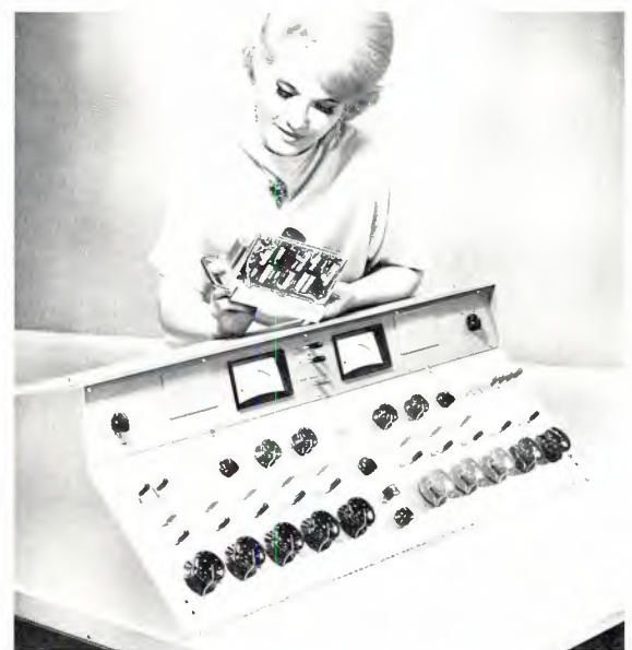
Plug-in chassis give flexibility to consolettes.
