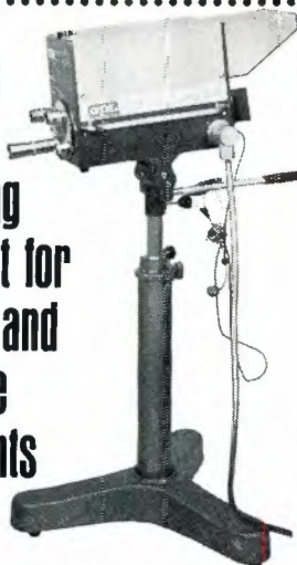
GENERAL PRECISION LABS Closed Circuit TV Camera on PS-34 Pedestal Stand with Model HD head. Model HD head features internal torsion spring to prevent camera dumping during extreme forward and backward tilts.
