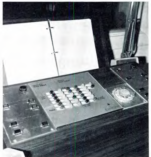
Fig. 7. Close-up of the flush-mounted call director unit.
