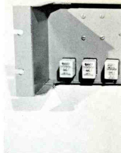
Rack mounted multiplexer showing placement of relays.
