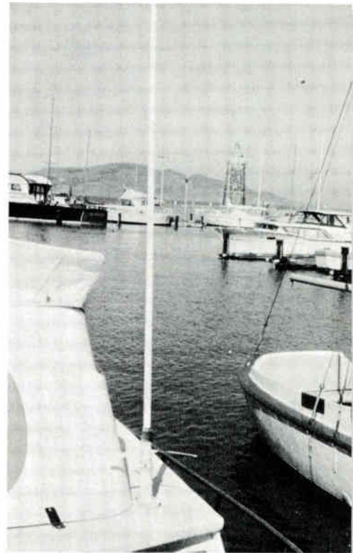
Location of deck mounted 450 MHz gain type antenna on marine cruiser.
