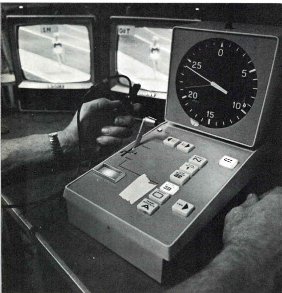
Dramatic Olympic action was recorded on HS-100 disc recorders from slow motion and stop action replay.
