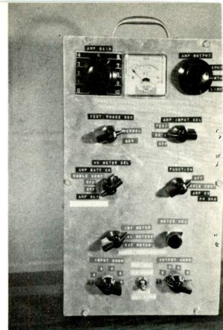
Fig. 5. Tester with VU meter, amplifier, speaker, ohmmeter and batteries built in.
