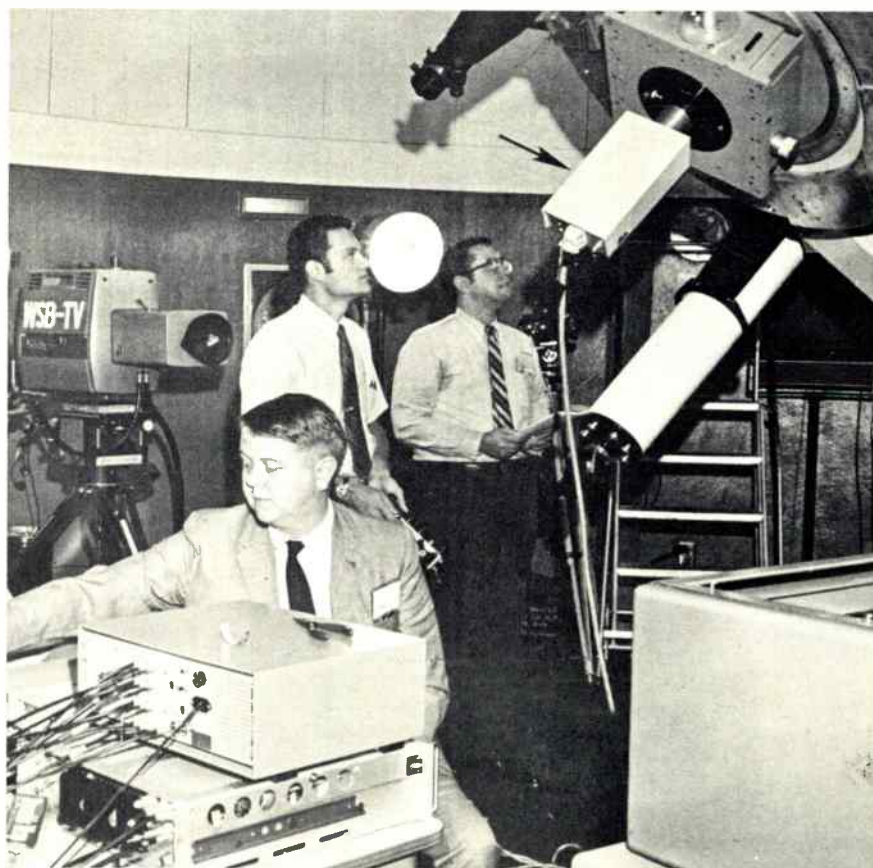
During Apollo 11, live television pictures of the moon were picked up through a 36-inch reflector telescope at Fernbank Science Center, Atlanta, Ga. using a small Norelco black-and-white TV camera (indicated by the arrow). Standing, center, is Fernbank astronomer Dr. Paul Knappenberger and to his left, Ralph Buice, acting director of the Chattanooga Satellite Tracking Station. Seated is Charles Irvin, systems specialist of Philips Broadcast Equipment Corp. WSB-TV in Atlanta handled the transmission of interviews and moon transmissions from the observatory for NBC.
