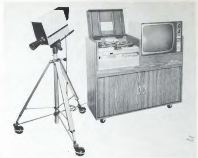
Fig. 3 This basic system includes a camera, videotape recorder, and monitor. Many major manufacturers are now offering origination packages to fit the needs of the low, medium and large budget system.
