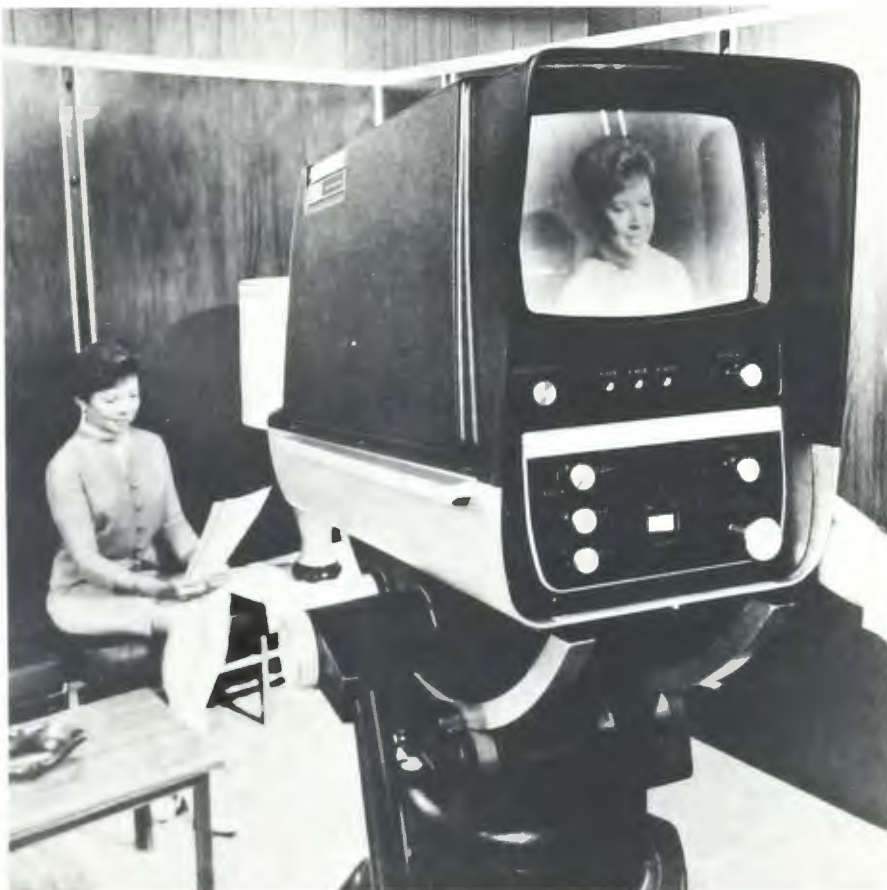
Fig. 12 Viewfinder cameras keep the cameraman from shooting blind.
