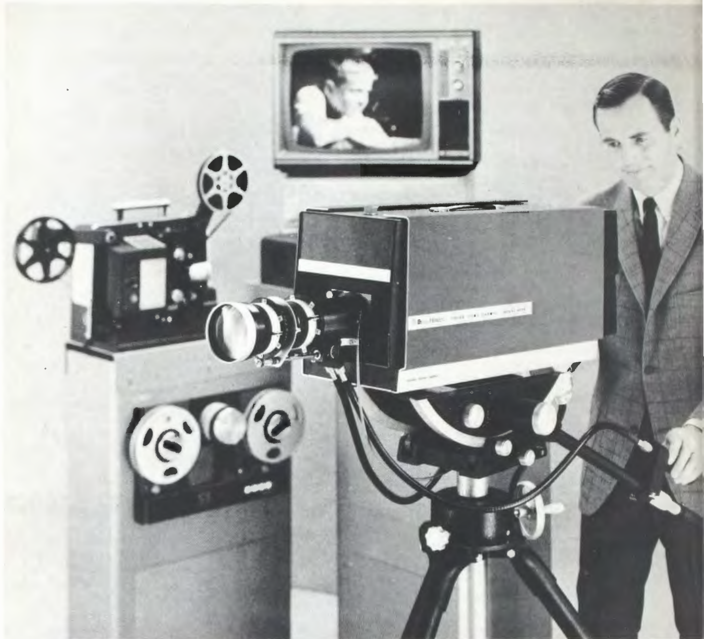
Fig. 7 This system arrangement allows the color camera to be removed from the film chain pedestal. With the addition of a standard zoom lens, it can be used for studio work.
