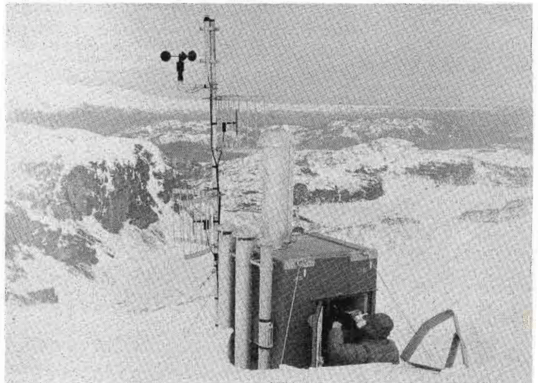
This is one of three 3M portable communications shelters which have undergone testing in Alaska.
