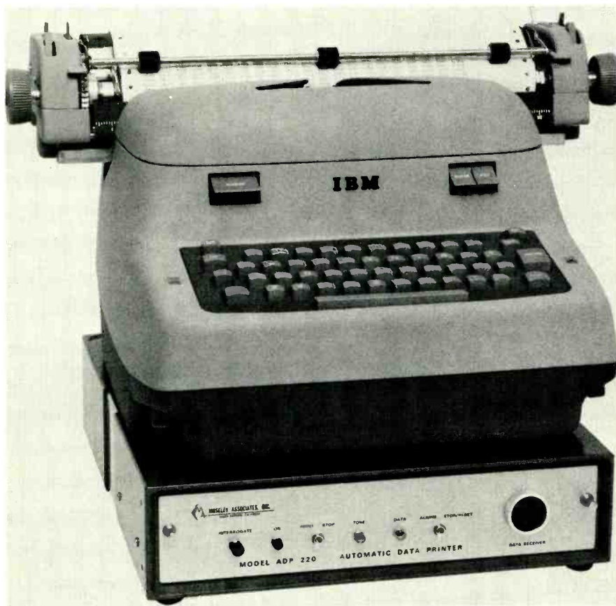
Fig. 4 The printout on this Moseley ADP 220 data printer is giving a record of equipment readings.
