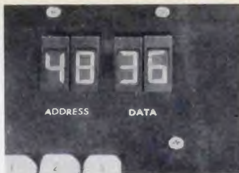
Fig. 5 The “seven segment” display. All numbers look square.
