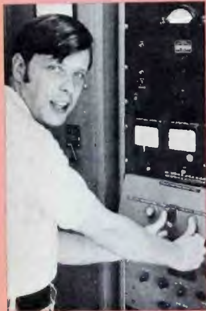
Fig. 1 The author is shown operating the panel. By pressing the appropriate button for power and mode change and then pressing the plate voltage reset button, the changeover can take place in less than one second.
