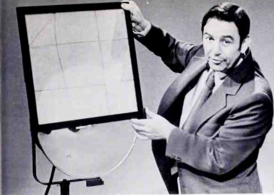
Fig. 1 Putting a spun glass filter on the scoop softens the light output, but it also reduces the light output by 33%.
