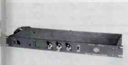
VIDEO AMPLIFIER WITH CLAMP, CHROMA CONTROL, AND SYNC-REFERENCED AGC
