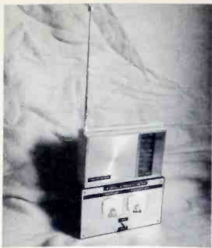
Fig. 1 The simple signal sampler built by the author includes meters for relative signal and modulation readouts.
