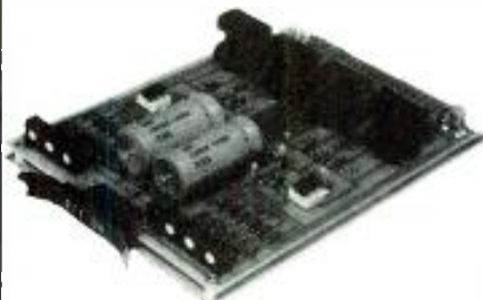
MODEL 211 1 x 6 DA, 6 differential source terminated outputs balanced within 1% $115.00
