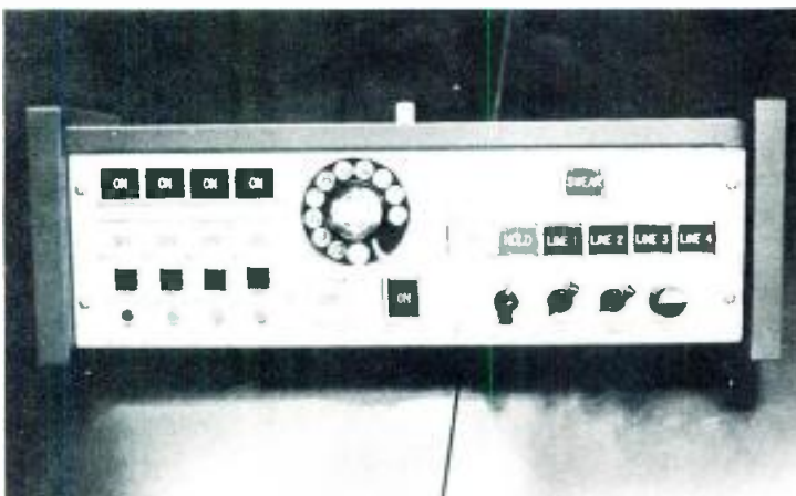
Fig. 2 Main switcher of the full-service system.
