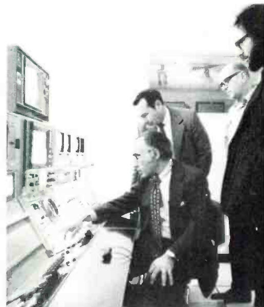
In the camera control area the author discusses switching routine. He is shown here checking burst, amplitude and phase with (L. to R.) Chief Engineer Joe Blake, maintenance tech Stan Macie, and Ross Kauffman, assistant Chief Engineer.
