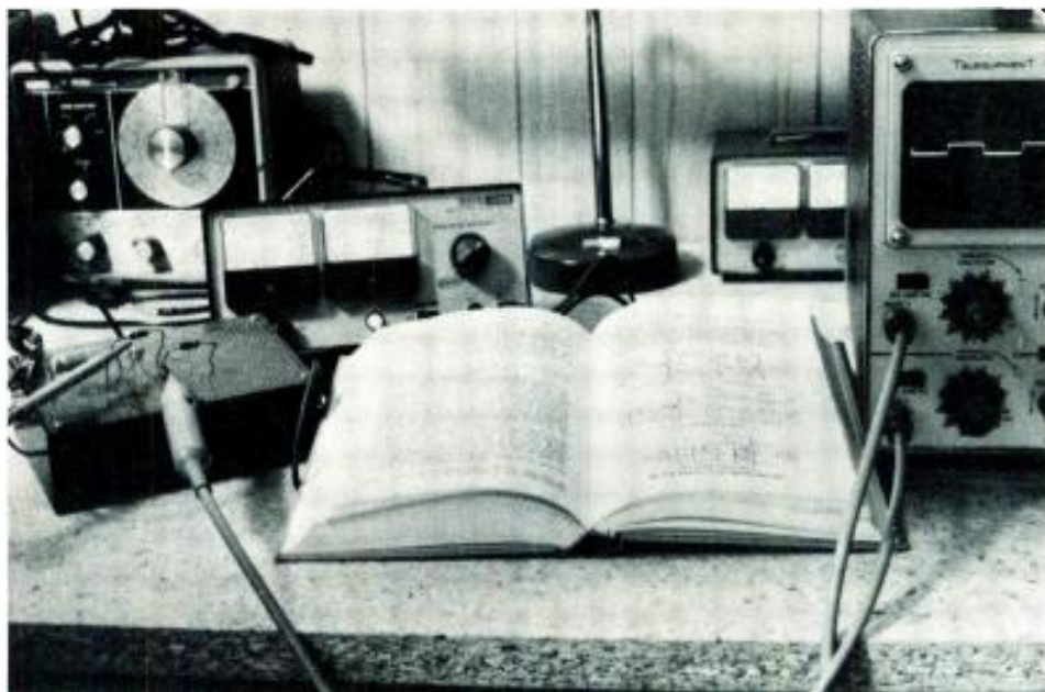
Fig. 2 A scope, variable power supply, breadboard and text make up essentials that should be available to the engineering staff for practical training on solid state circuits and, especially, IC's and IC logic.
