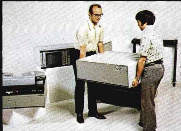
All components are light enough so that two men can disassemble and move AVR-2 in minutes.
