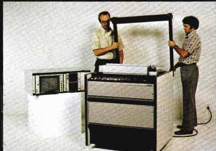
All components are light enough so that two men can disassemble and move AVR-2 in minutes.
