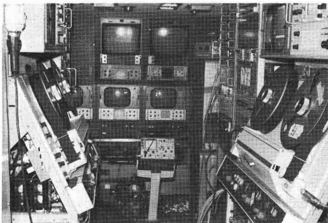
This is a tight view inside the Olympic van, including two VTR's and complete switching and video monitoring.
