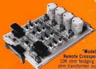
Model 227 4X1 Remote Crosspoint Switch 600 ohm transformer inputs. 600 ohm bus output. TTL, CMOS, compatible DC control. Unity to +10 dB gain adjustment.
