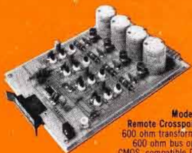
*Model 223 6X1 Active Mixing Network 10K ohm differential inputs/50 dB CMR. 600 ohm output. Individual input level controls. Unity to +20 dB gain adjustment. 60 dB/400 Hz channel isolation.
