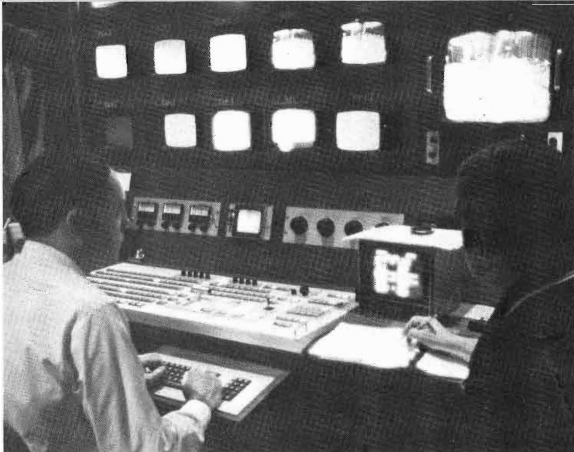
Fig. 1 Engineer, Carl Erny (left) and Director, Mike Andrews enter data from the program schedule via the local keyboard into the system. (All photos by Myles Marks.)
