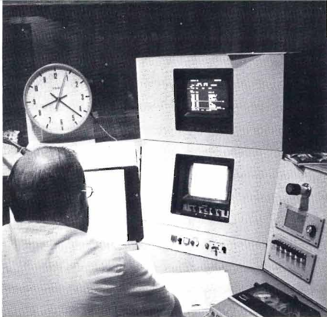
Fig. 2 Computer status read-out monitor in the announcer's booth is located above the on-air picture monitor, aiding the announcer to determine when he will receive cues.
