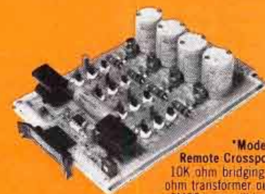
Model 227 4X1 Remote Crosspoint Switch 600 ohm transformer inputs. 600 ohm bus output. TTL, CMOS, compatible DC control. Unity to +10 dB gain adjustment.
