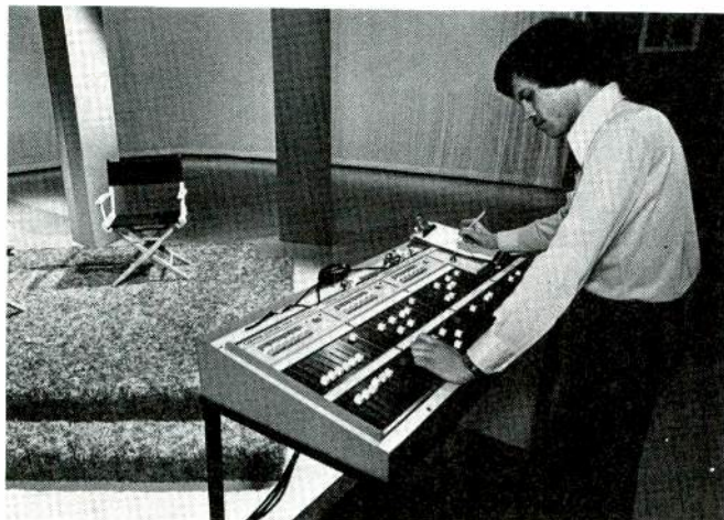
With the dimmer control panel mounted on a mobile stand, the board can be moved to any location for close in viewing of lighting adjustments.
