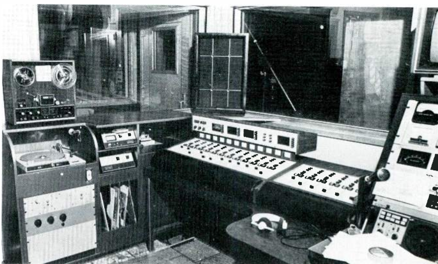
The actual changeover time to this new setup was only three and a half hours. Step by step planning included the console desk, utility cabinet for record and tape equipment, and turntable cabinet.
