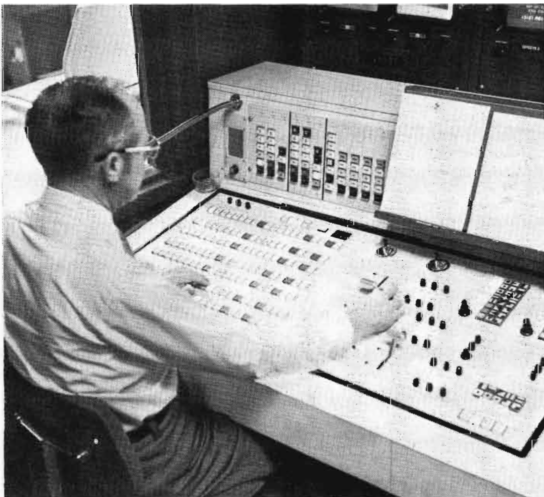
Cue On-Off buttons are on the main console on the top row.
