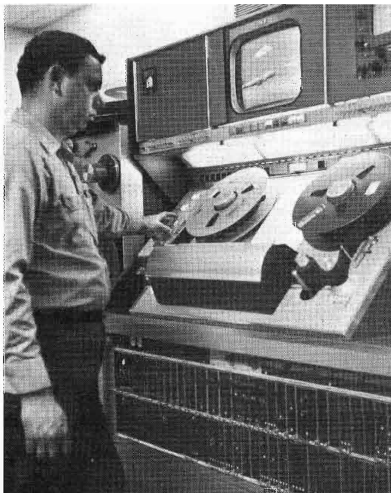
John Brewer hits the cue tone button on the VTR. He's cueing tapes for KSLA-TV news.
