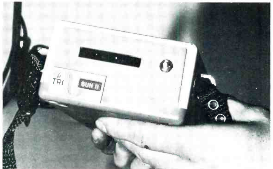
This Sun II portable time code generator can be slung over the operator's shoulder and provide the SMPTE address code for remote recordings.
