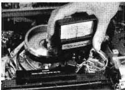
Shown measuring the critical supply tension on a Sony 2850
