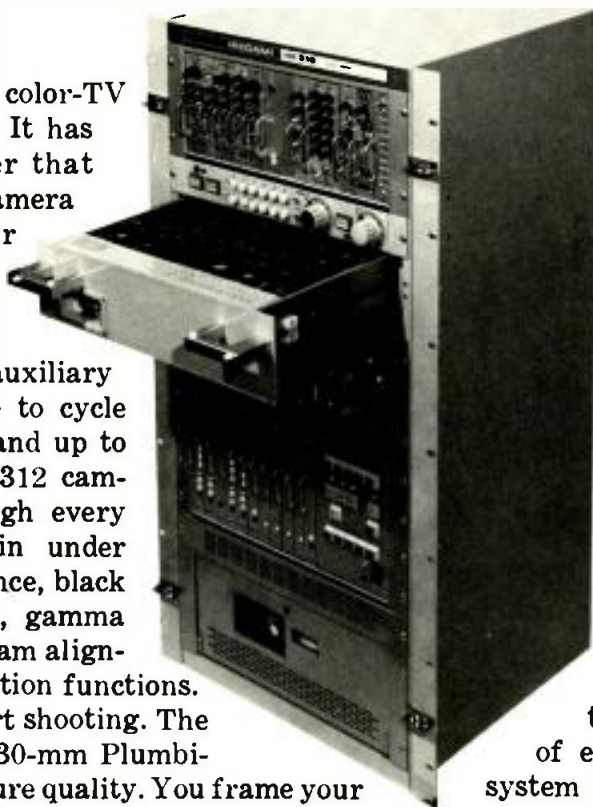
Camera-control unit for the HK-312
