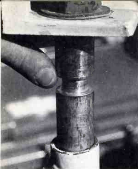
Two, one-inch pipe nipples 12 inches long and four, one-inch floor flanges are used to construct the lamp mounts. See text for complete instructions.
