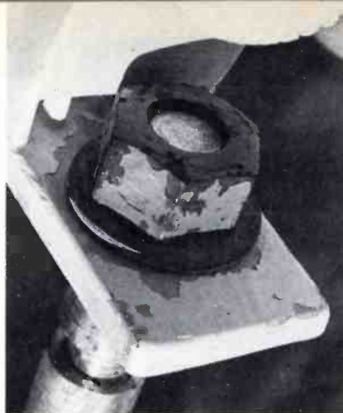
Two, one-inch pipe nipples 12 inches long and four, one-inch floor flanges are used to construct the lamp mounts. See text for complete instructions.
