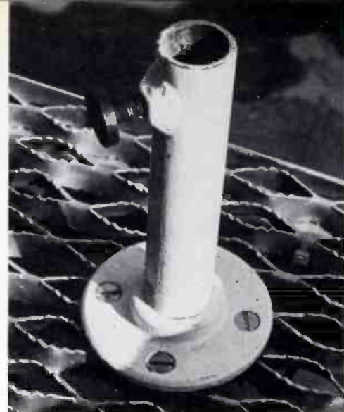
Two, one-inch pipe nipples 12 inches long and four, one-inch floor flanges are used to construct the lamp mounts. See text for complete instructions.
