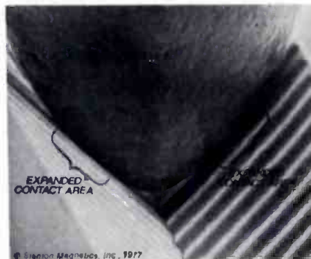
Scanning Electron Beam Microscope photo of Stereohedron Stylus, 2000 times magnification.
