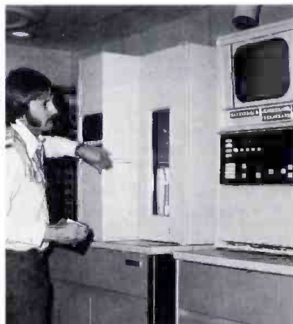
A technician at KTVQ-TV finishes loading cassettes into the station's Ampex ACR-25 videocassette recorder in preparation for the broadcast day.
