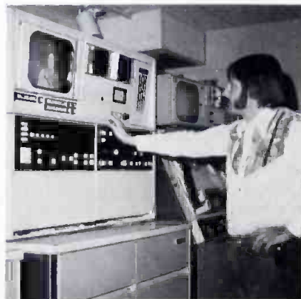
A technician at television station KTVQ-TV previews a cassette on the station's Ampex ACR-25 videocassette recorder. The station uses the recorder to broadcast 300 to 400 cassettes during a typical broadcast day.
