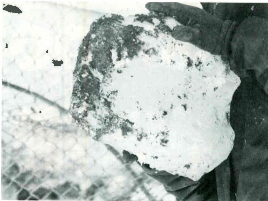
This chunk of ice was recovered from the tower leg. Other chunks of ice bearing the imprint of the leg were found that weighed between 30 and 40 pounds.
