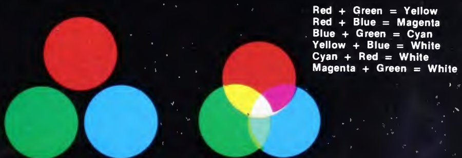
Figure 3. For color TV the primary colors are red, green and blue. A wide range of colors are possible by mixing of the primaries, with white being an equal mixture of all three.
