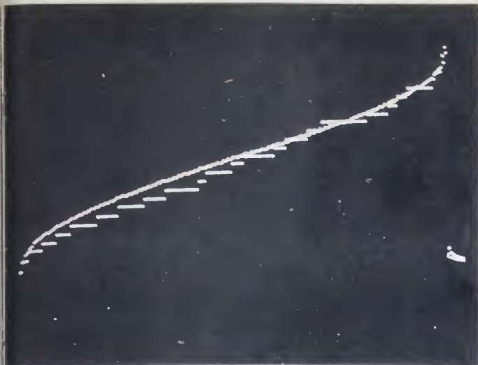
Figure 7. Co-channel beat with skywave setting in (note rag on left).
