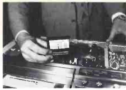
Wayne Graham, Tentel, demonstrates their unique tape tension gauge for in-line measurements on audio and video recorders. (C. Cave)
