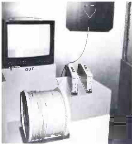
Bosch-Fernseh displayed its fiber optics laser link for video and audio transmission. (C. Cave)
