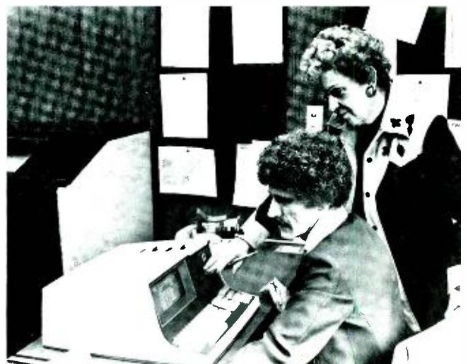
Traffic manager Jack Winslow and Virginia Lane enter the WWDL-FM log into the BAT system desktop minicomputer. The next step will be to dump the entire day's program into the System 7000 memory.
