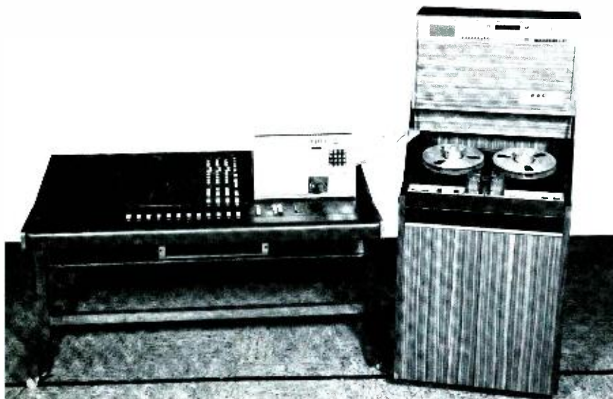
Figure 3 BBC Research Department's 10-channel digital audiotape recorder was digitally coupled to an experimental digital mixing console, based on a Plessey Miproc computer. The recorder is the forerunner of the 3M/BBC multi-channel recorder.
