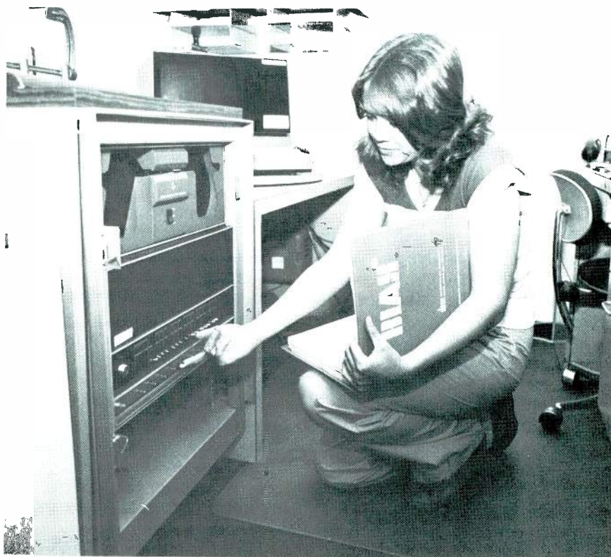
In the KOMO-TV traffic department, Claudia Whipple resets controls on the Data General Nova 2 minicomputer system following the BIAS documentation.
