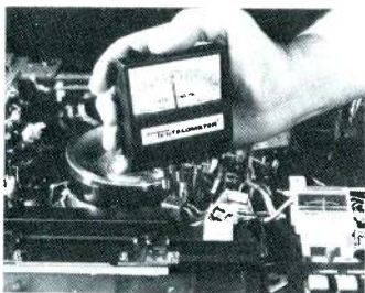
The T2-H15-UM TENELOMETER® Tape Tension Gage shown checking the critical hold-back tension on a Sony 2850. Price $225 complete.
