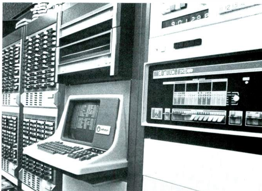
Figure 2 The 770 programming and switching automation system forms one branch of the CBS Radio instrumentation package. More than seven full days of programming may be stored. The disc cartridge unit immediately above the Infotron terminal provides massive data storage and rapid data access.
