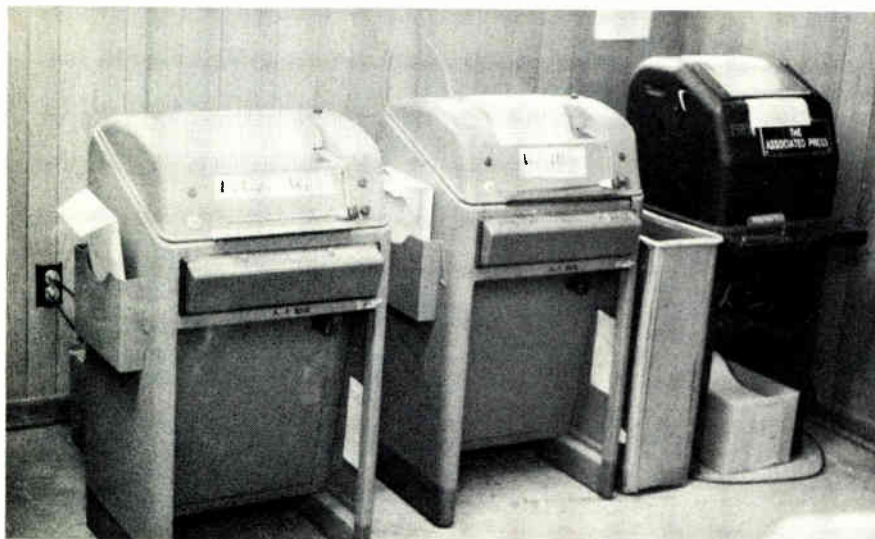
Fig. 3 Note that police, weather and radio wire machines are not jammed together. The other machines are a different type that do not require a far forward paper box position.
