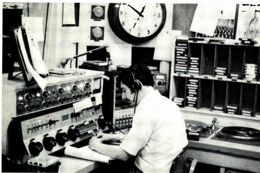
Fig. 1 KPRS Kansas City has set up their radio wire room just seconds away from the DJ's position at the console. Also, note that there are bulletin warning lights to the left of the clock.
