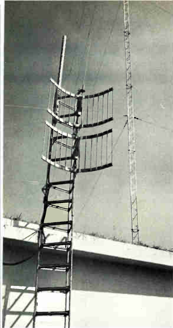
Fig. 3 The 450 MHz transmit and receive antennas for Civil Defense communications. Baseball bat type antenna is used on 455.85 MHz for AM programming.
