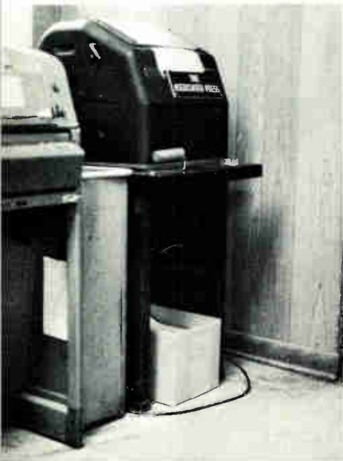
Fig. 2 Forward edge of the paper supply box should come directly under the front shelf.
