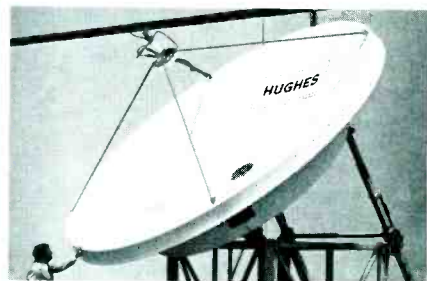
Hughes: Antennas have dual-polarized feeds for choice of focal point or prime focus feeds.
