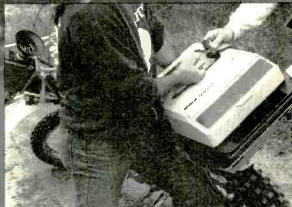
The Bosch BCN 20 portable 1" recorder, weighing only 44 lbs., provides images with multiple generations superior to quad.
