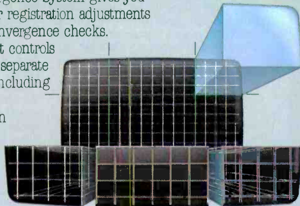
Conrac's Active Convergence system lets you adjust color registration on nine separate areas of the CRT.
