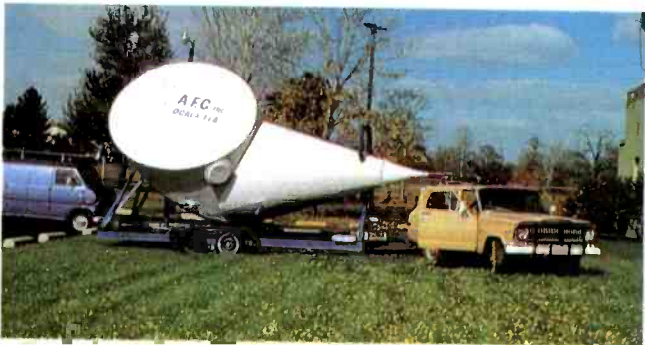
Mobile earth station at Network Operation Center for the network interconnection with PBS.
