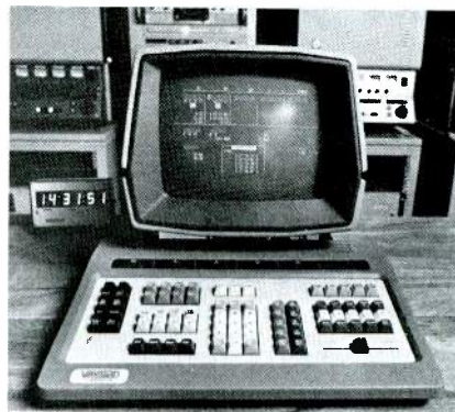
This is a closeup view of the Vanguard keyboard and CRT display.
